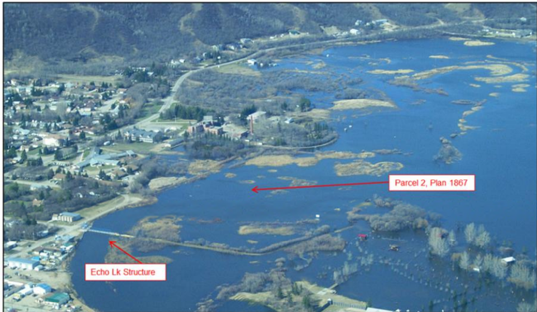
Photo date is May 3 rd , 2011. Water level is approximately 480.89 m elevation. 1:100 year calm is 480.9 m & 1:500 year calm is 481.4 m.
